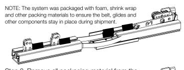
Step 2. Remove all packaging material from the Track, ensuring the Drive Belt stays in place inside the Track.
