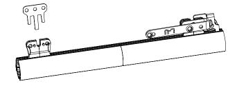
Step 5. Tighten the Splice set screws.
