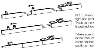
NOTE: Keep the Drive Belt tight and straight inside the Track as the Master Carrier is pushed forward.
