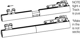
NOTE: Keep the Drive Belt tight and straight inside the Track as the Master Carrier is pushed forward.
