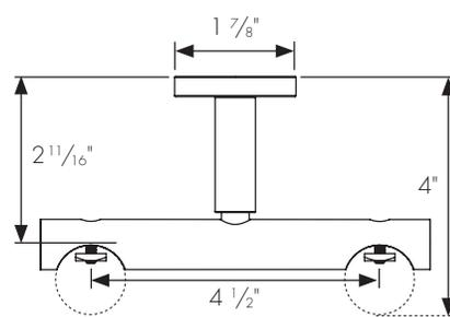
1<sup>3</sup>/<sub>8</sub>" metal ceiling bracket extender
