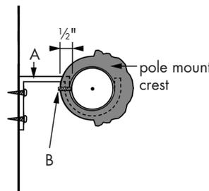
Set screw (B) holds crest in place. Be sure the return (distance from wall to center of cradle) on your pole brackets (A) allow the back of the crest to clear the wall and other objects.
