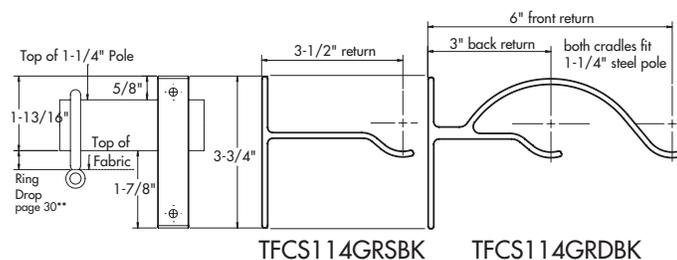
Bracket return measured from wall to center of cradle.
