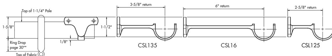
Bracket return measured from wall to center of cradle.
