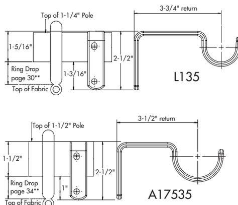
Bracket return measured from wall to center of cradle.
