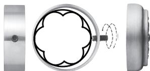
Attach any rosette to the front of a pole. Metal band slides onto pole and is locked in place with set screw. Set screw should be positioned in the front center of pole because it receives the rosette. Rosettes sold separately.
