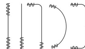
Please note: Somfy Glydea® systems can be curved with a minimum 11.8" radius. All curves require a template. Curving track reduces weight capacity of motor. Please refer to motor specifications above.
