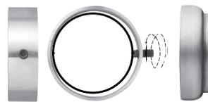
Metal band slides onto pole and is locked in place with set screw. Set screw should be positioned in the front center of pole because it receives the rosette.
