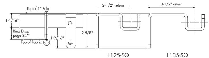
Bracket return measured from wall to center of cradle.
