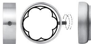
Metal band slides onto pole and is locked in place with set screw. Set screw should be positioned in the front center of pole because it receives the rosette.
