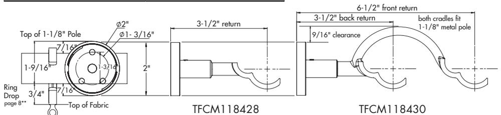
Bracket return measured from wall to center of cradle.
