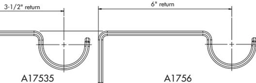
Bracket return measured from wall to center of cradle.
