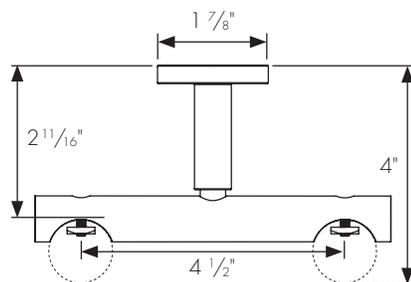
1<sup>3</sup>/<sub>8</sub>" metal ceiling bracket extender
