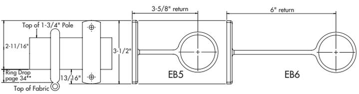
Bracket return measured from wall to center of cradle.
