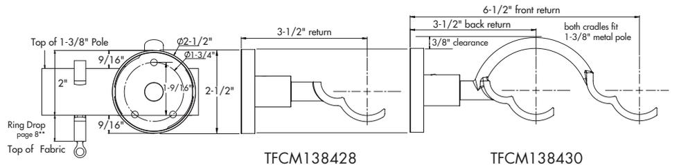
Bracket return measured from wall to center of cradle.
