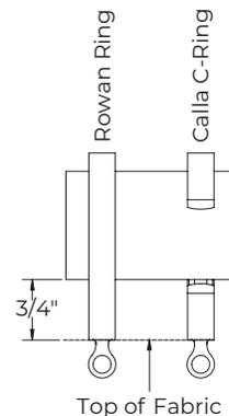
Note: Ring drop indicates distance from bottom of pole to bottom of ring. A ring's drop changes on different diameter poles. \*\*
