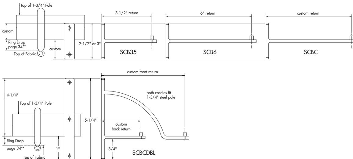
Bracket return measured from wall to center of cradle.
