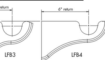
Bracket return measured from wall to center of cradle.
