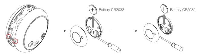
Replace cover by aligning notches and press together.
