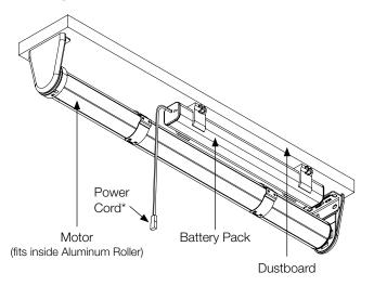
\*Power Cord plugs into the Motor from the Battery Pack. Keep cord away from rotating parts of the shade during operation.
