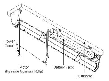
\*Power Cords plug into each other from the Motor to the Battery Pack. Keep cords away from rotating parts of the shade during operation.
