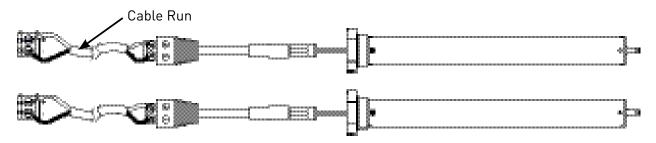
This connection may only be used when wiring 28mm & 25mm motors to the distribution panel, as these motors do not exceed the 1.33 A current limit per channel.
