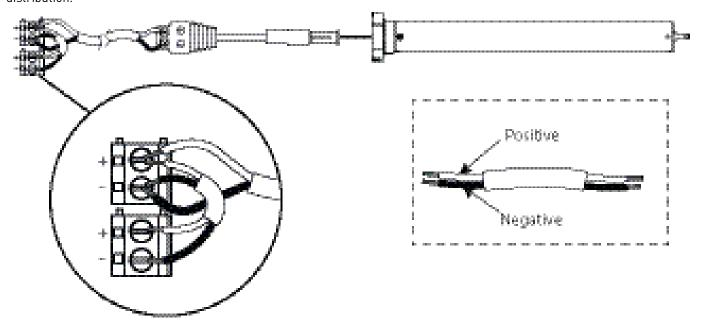
Due to 1.33A limit per channel, working current can be doubled to 2.66A with parallel configuration as shown above, allowing connection of 45mm and 35mm motors.
