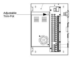
If motors powered by the DC Power Distribution Panel are to be used with the R-TEC AUTOMATION® HUB & APP, the output voltage of the Distribution Panel **MUST** be adjusted to allow for proper communication between the Hub and Motor.
