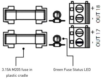
In order to replace fuse, carefully pry the fuse out of the plastic cradle using a small tool (such as a small screwdriver or pen). To replace, gently press the new fuse into the cradle.
