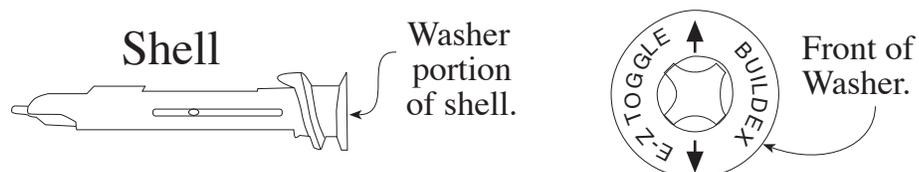
Step 2) So the screw does not thread incorrectly inside the shell, be sure to slightly angle the screw from the direction show below.
