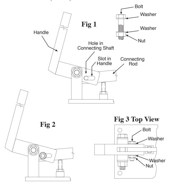
Remove the nut and only one plastic washer from the bolt.
