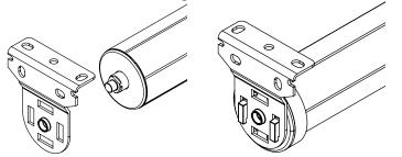
Figure 11A. End Pin Bracket
