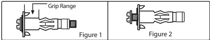
Step 2: Back the screw head out until the end of the screw is even with the end of the anchor. See Figure 2.
