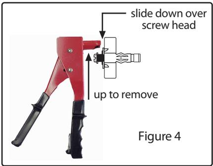
Step 5: To mount bracket: Remove screw and place through the hole in bracket. Re-insert screw in anchor shell in wall and only tighten until all pieces come together snugly. Do not overrun.
