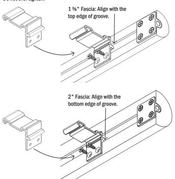
10. Lift the track assembly onto the wall brackets and secure in place.
