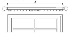
Cut the fascia to the required length. The fascia should be cut to the dimension (x). For example, if you want a 48" drapery, the fascia should be cut to a length of 48". Use a fine tooth wood saw to cut the fascia.
