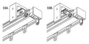
11. Hook the fascia clips over the back of the track and push down on the top of each of the clips until all the clips snap into place. The fascia should overhang each end of the track assembly by 1/8".
