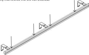
9. Attach the fascia clips at your marked locations onto the back of the wood fascia as shown below. Align the front locating tab on the fascia clip to the top edge of the slot when using a 1 %" fascia. Align the front locating tab on the fascia clip to the bottom edge of the slot when using a 2" fascia. Pre-drill the holes with the 3/32" drill bit so the fascia won't split and use the screws provided to secure the clip to the wood fascia. Do not over tighten.
