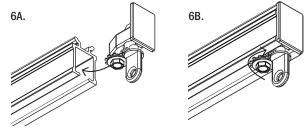
7. Attach the wall mounting brackets. Use two brackets at each end of the track no more than 24" apart. Then place brackets no more than 48" apart over the remainder of the track. Securely attach all brackets to the mounting surface. Mount brackets to wall studs whenever possible. Use proper fasteners designed for your particular type of mounting surface. Hollow wall fasteners (sold separately) are recommended for dry wall. Use a level to make sure all brackets are lined up.
