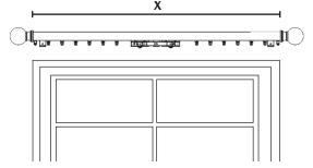
Cut the fascia to the required length. The fascia should be cut to the dimension (x). For example, if you want a 48" drapery, the fascia should be cut to a length of 48". Use a fine tooth wood saw to cut the fascia.
