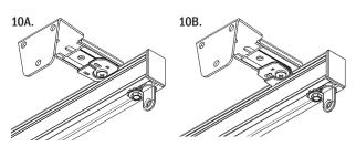
11. Hook the fascia clips over the back of the track and push down on the top of each of the clips until all the clips snap into place. The fascia should overhang each end of the track assembly by 1/8".
