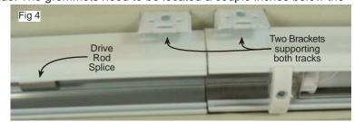
**Splicing Headrail:** See fig 4. Use our Drive Rod Splice to join the Drive Rod together. No splice is needed to join the Headrail but you will need to adequately support both ends of the headrail with a separate bracket on each end. The brackets should be no more than two inches apart. Try to position the splice so it carries the least amount of weight by locating it as far as possible from the clutch.
