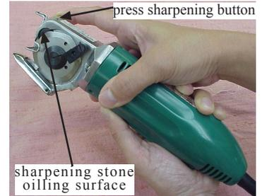
Figure 2. Blade Sharpening
