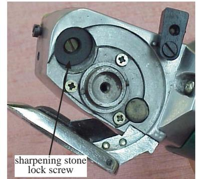
Figure 5. Sharpening Stone
