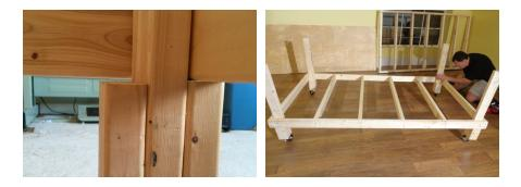
For the bottom shelf plywood, cut out corners for legs, then screw to bottom frame, all the while checking for square.
