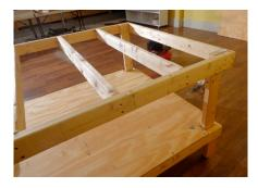
Place the two pieces for the top, measuring to ensure a 2" lip on all four sides. Mark support board placement for easy screwing. Screw down top.
