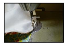
Turn bolster, right sides out, insert pillow form, and hand stitch the opening closed to complete the bolster.
