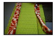
Determine the placement for the grommets and mark on the contrast band. Cut grommet holes in band. Set grommets in band being sure to catch the folded in sides in the grommets.
