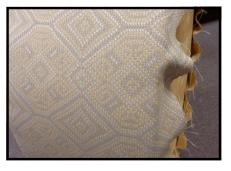
Staple the fabric to the prepared frame so 3" is above the top – to wrap to the inside – and 2" to staple to the bottom.
