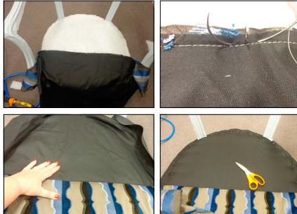
At the front corners, make a peace sign relief cut and fold around leg. Trim, fold under and staple.
