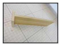
**C.** For the dust board, Use wood if making a large cornice. Wood was used in this sample. Sample was 81"L x 4"W x 2"thick.
