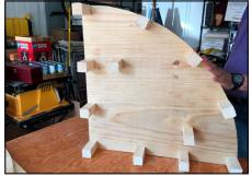
Measure and mark for T-Nut placement.
