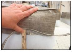
Using cardboard tack strip, put on the bottom banding, making a join at a corner, aligning it with a boxing join.
