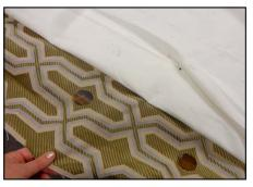
Set grommets on a diamond, assuring placement is accurate to pattern motif.
