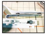
If using an exposed baton, place the empty Stiffener in the Master Carrier arm. Hold the tape to the Stiffener to mark where the tape needs to end (tape should butt up next to the stiffener). Cut the tape to length and staple to hold in place.
