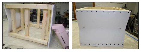
Lay the open side down on a larger piece of FirmaFlex™ and trace around it for the sides.
