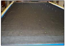
Lay shroud cord alongside of pins and tack at each pin.
