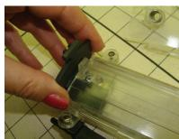
3. Slide out the pick-off at the end of the pinsetter.
