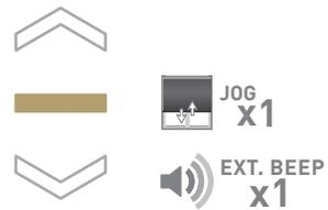
If motor is in Step Mode, use following steps to change to Roller Mode
