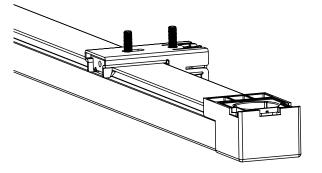
NOTE: To release track, push release lever.
