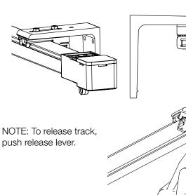
Step 5. Install End Hook on both Drive Pulleys.
