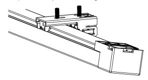
Step 4. Push system upward until system clicks in place.
