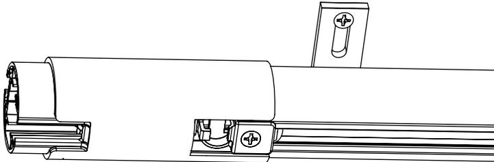
NOTE: Glides can be added or removed with the Drive Pulley installed by removing the End Stop.
