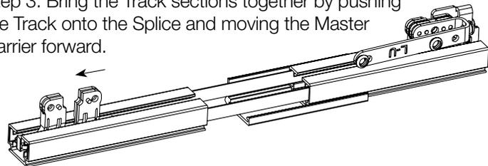
Note: Keep the Drive Belt tight and straight inside the Track as the Master Carrier is pushed forward.\*Make sure the belt remains in the track channels and is not pinched as the splice sections move forward.
