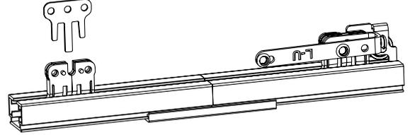
Step 5. Tighten the Splice set screws.
