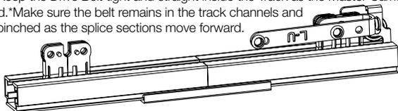
Step 4. Bring both Master Carrier Body halves together and insert the center clip.
