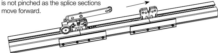
**Step 4.** Bring both Master Carrier Body halves together and insert the center clip.
