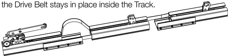
**Step 3.** Bring the Track sections together by pushing the Track onto the Splice and moving the Master Carrier forward.
