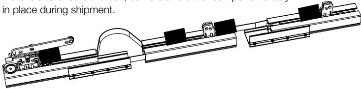
**Step 2.** Remove all packaging material from the Track, ensuring the Drive Belt stays in place inside the Track.
