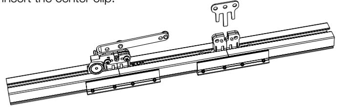
**Step 5.** Tighten the Splice set screws.
