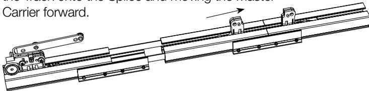
**Note:** Keep the Drive Belt tight and straight inside the Track as the Master Carrier is pushed forward.\*Make sure the belt remains in the track channels and is not pinched as the splice sections move forward.
