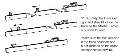
Step 4. Bring both Master Carrier Body halves together and insert the center clip.
