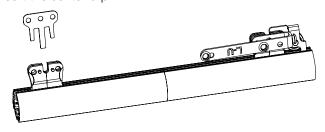
Step 5. Tighten the Splice set screws.
