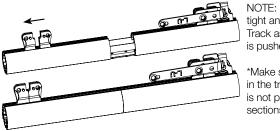
NOTE: Keep the Drive Belt tight and straight inside the Track as the Master Carrier is pushed forward.
