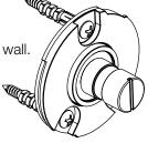
Step 3. Locate bracket base cover. Place cover over wall mount base plate. Turn cover clockwise to lock in place.
