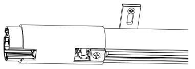
NOTE: Carriers can be added or removed with the Drive Pulley installed by removing the End Stop.
