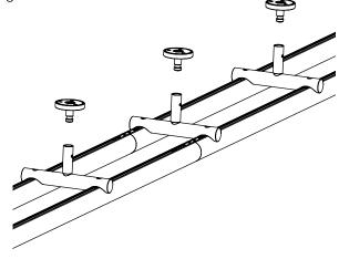
Step 6. Tighten all ceiling mount stems with set screw located close to the ceiling mount cover.
