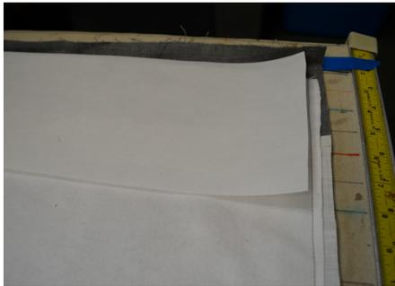
11 Turn the panel right side out, press the lead edge with the seam right on the edge. Fold the return side hem and hem in your method of choice.
