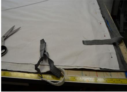
10 Place buckram on interlining, glue baste or use iron on bonding tape to keep in place.
