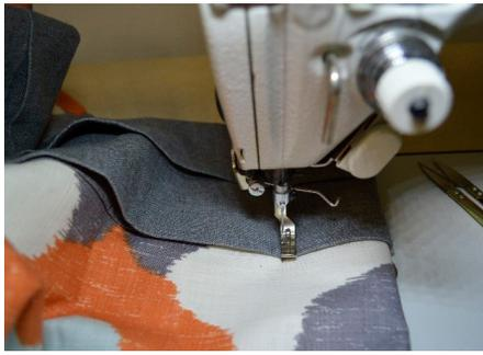
14 Prepare the trim for the panel lead edge. Sew two rows of the trim together along the outer edge.
