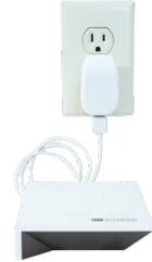
5. Plug the Power Supply into the outlet and place the Hub in a central location in your home.
