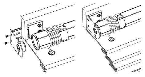
10. The shade assembly is complete at this point and can be installed onto the wall or ceiling per your preferred method (Angle Brackets, Z Brackets, Direct Attachment, etc.). Make sure the shade assembly is level when installed to ensure the shade operates properly. After the shade is mounted, test the operation by raising and lower a couple of times. Continue on to steps 10 and 11 if you need adjust the spring tension or the up stop position.
