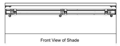
7A. To release the locking mechanism in the spring, the roller tube assembly must rotate roughly ¼ turn, which allows the spring to release and raise the shade. To allow the spring to release, you must have extra travel distance in the fabric at the bottom of your shade to pull the shade down and release the spring.
