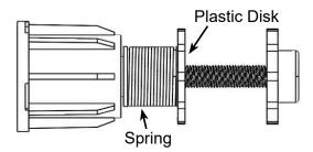
4B. Line up the grooves on the length adjuster to the matching ribs on the roller tube.
