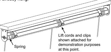
6B. Front or Waterfall Mount: Lift cords off the front of the roller tube assembly.
