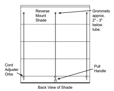
7B. With the shade laying on a flat surface, use your hands to roll the lift cord onto the roller tube assembly like you were raising the shade. Stop rolling once you get to the where you want the shade to stop in the up position.
