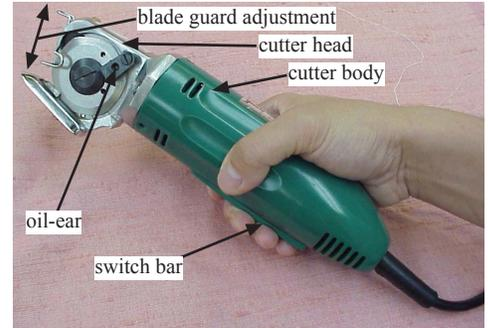
Figure 1. Electric Rotary Cutter
