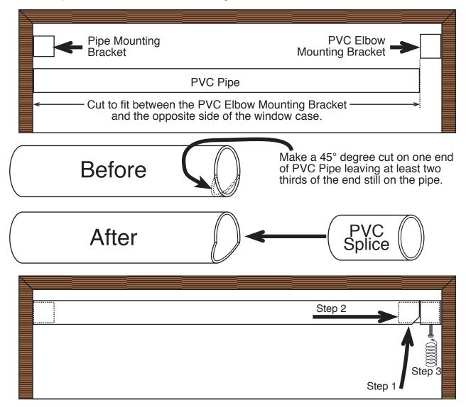
If fabric is to be shirred onto the pipe, do so now. Place a PVC Splice into the angled end of the pipe and swing the end up and in line with the Elbow Mounting Bracket. Hold in place and use your thumb to push the PVC Splice into the Elbow Bracket. Secure the pipe by running a screw through the bracket into the splice.
