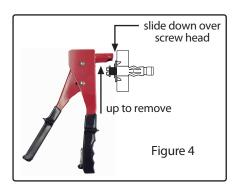
Step 5: To mount bracket: Remove screw and place through the hole in bracket. Re-insert screw in anchor shell in wall and only tighten until all pieces come together snugley. Do not overrun.
