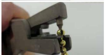
**Step 4** Partially open one end of the chain (left), but completely open and remove the ball on the other end of the chain (right).
