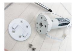
B. Slide the crown onto the battery tube, lining up the notch and grooves.
