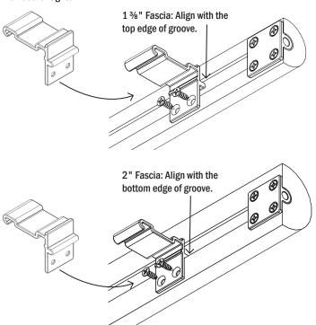
10. Lift the track assembly onto the wall brackets and secure in place.
