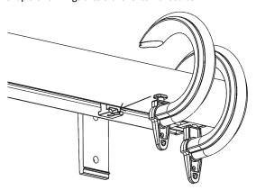
15. Install the finials onto both ends of the wood fascia by screwing the finials into the fascia clips. Tighten the finial until it contacts the track end cap.
