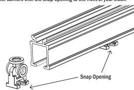
Install the end caps onto the track. (One side shown - repeat for the other side).
