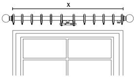
Cut the fascia to the required length. The fascia should be cut to the dimension (x). For example, if you want a 48" drapery, the fascia should be cut to a length of 48". Use a fine tooth wood saw to cut the fascia.
