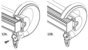
13. Lift the track assembly onto the wall brackets and secure in place.
