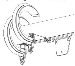
15. Install the finials onto both ends of the wood fascia by screwing the finials into the fascia clips. Tighten the finial until it contacts the track end cap.
