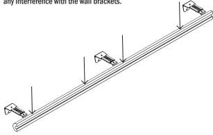
9. Attach the fascia clips at your marked locations onto the back of the wood fascia as shown below. Align the front locating tab on the fascia clip to the top edge of the slot when using a 1 % " fascia. Align the front locating tab on the fascia clip to the bottom edge of the slot when using a 2 " fascia. Pre-drill the holes with the 3/32" drill bit so the fascia won't split and use the screws provided to secure the clip to the wood fascia. Do not over tighten.
