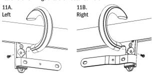
Attach the "C" Rings onto both end caps. (One side shown - repeat for the other side).
