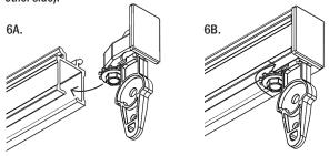
Tips for Successful Installation Securely attach all brackets to the mounting surface. If you do not locate and install into wood studs, use the proper wall fasteners and/or plastic anchors designed for your particular mounting surface (screws and plastic anchors not included). When drilling into metal, use self-tapping screws (not included).
