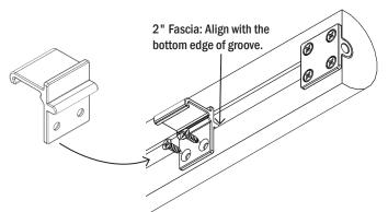
10. Hook the fascia clips over the back of the track and push down on the top of each of the clips until all the clips snap into place. The fascia should overhang each end of the track assembly by 1/8".
