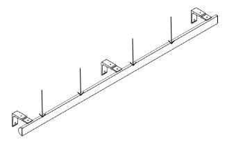
3. Attach the fascia clips at your marked location onto the back of wood fascia as shown below (3A). Align the bottom of the fascia clip with the bottom edge of the wood fascia (3B). Pre-drill the holes with a <sup>3</sup>/<sub>32</sub>" drill to keep the fascia from splitting. Use the screw provided to secure the fascia clip to wood fascia. Do not over tighten.
