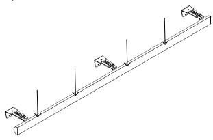
Attach the fascia clips at your marked location onto the back of wood fascia as shown below (3A). Align the bottom of the fascia clip with the bottom edge of the wood fascia (3B). Pre-drill the holes with a  $^3/_{32}$  " drill to keep the fascia from splitting. Use the screw provided to secure the fascia clip to wood fascia. Do not over tighten.
