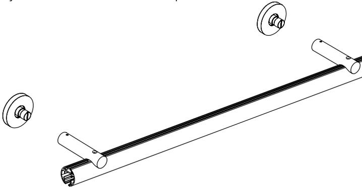
Step 5. Tighten all wall mount stems with set screw located above the wall mount cover.
