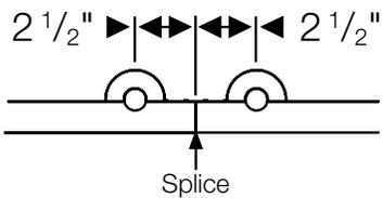
Step 2. Locate the splice and install it in the track sections. Line up both track sections and tighten the set screws.
