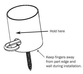
8. Locate the Finial Wall Mount Adaptor screw and mount assembly to the wall, as shown below.
