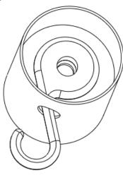
Attach the Finial Wall Mount Adaptor to the wall by holding Finial Wall Mount Adaptor assembly above the hook hole location.
