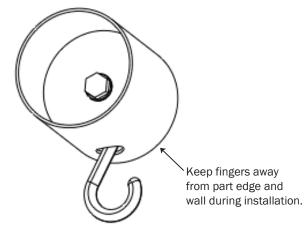
Assemble the Finial (Sold Separately) to the Finial Wall Mount Adaptor by placing the finial over the 1 <sup>3</sup>/<sub>8</sub>" pole. To secure the finial to the pole tighten the 4 mm set screw to the pole.
