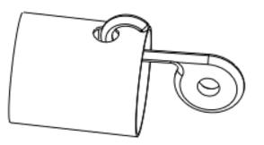
5. Then rotate the hook and 1  $\ensuremath{\$}\sp{\$}"$  pole until both holes line up as shown below.
