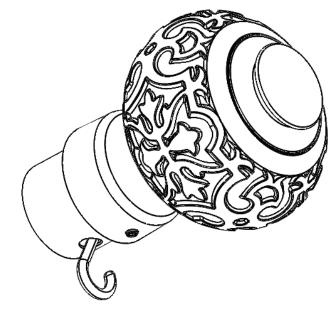
6. To install the mount screw, place it through the center of the 1  $^1\!/_2"$  pole & the optional hook, as shown below.
