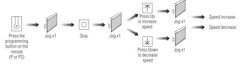
Note: If motor doesn't jog, the max/min speed has already been reached. Motor has 3 adjustable speeds.
