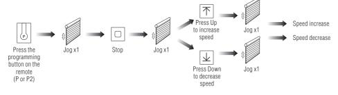
Note: If motor doesn't jog, the max/min speed has already been reached. Motor has 3 adjustable speeds.
