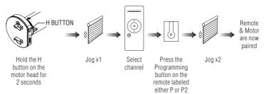
Note: A maximum of 15 motors can be added to one channel. All motors added to the same channel will operate simultaneously
