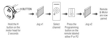
Note: A maximum of 15 motors can be added to one channel. All motors added to the same channel will operate simultaneously
